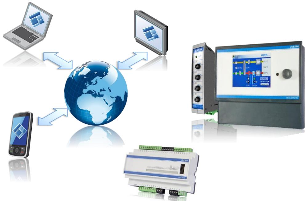
The Web-Server provides the visualization and operation of plant data and alarms with a standard Web-Browser. With the help of the Web-Browser every PC becomes an operator terminal. The installation can be accessed at any time directly at the control panel or via Intranet or remote via the Internet.
