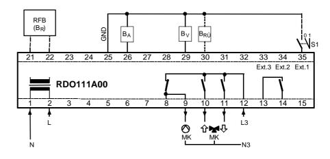
**2-point mixing valve-heating circuit** (with or without limitation of return temperature) (without return sensor: pump "KK" and bypass are not necessary)
