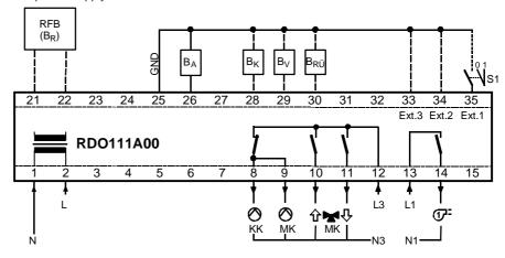
S1: External "() "Standby" controller (boiler and heating OFF)
