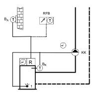
Direct boiler-heating circuit, Burner 1 stage
