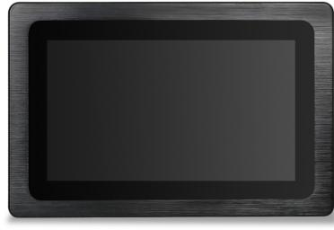
The Controlesta RCO 695D-S is a graphical 15,6" touch operator panel for the building automation system Controlesta RCO. The operator panel connects to the embedded web server of a controller of the RCO 8...D-W, RCO9...D-W series over the TCP/IP network. Animated visualizations for graphical operation, setpoints, time schedules, etc. can be changed, trends can be visualized, alarms are displayed and can be acknowledged.
