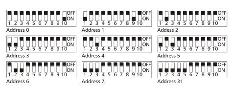
DIP switch 1-5: Address 0-31 adjustable DIP switch 6-7: Without function
